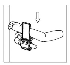
Press the handle clip down by arm to open/ close the door.
