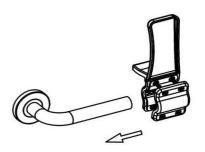
3. Put the handle clip from the end of the lever handle and tighten the screws.
