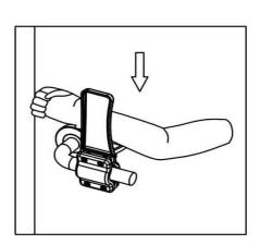
Press the handle clip down by arm to open/ close the door.
