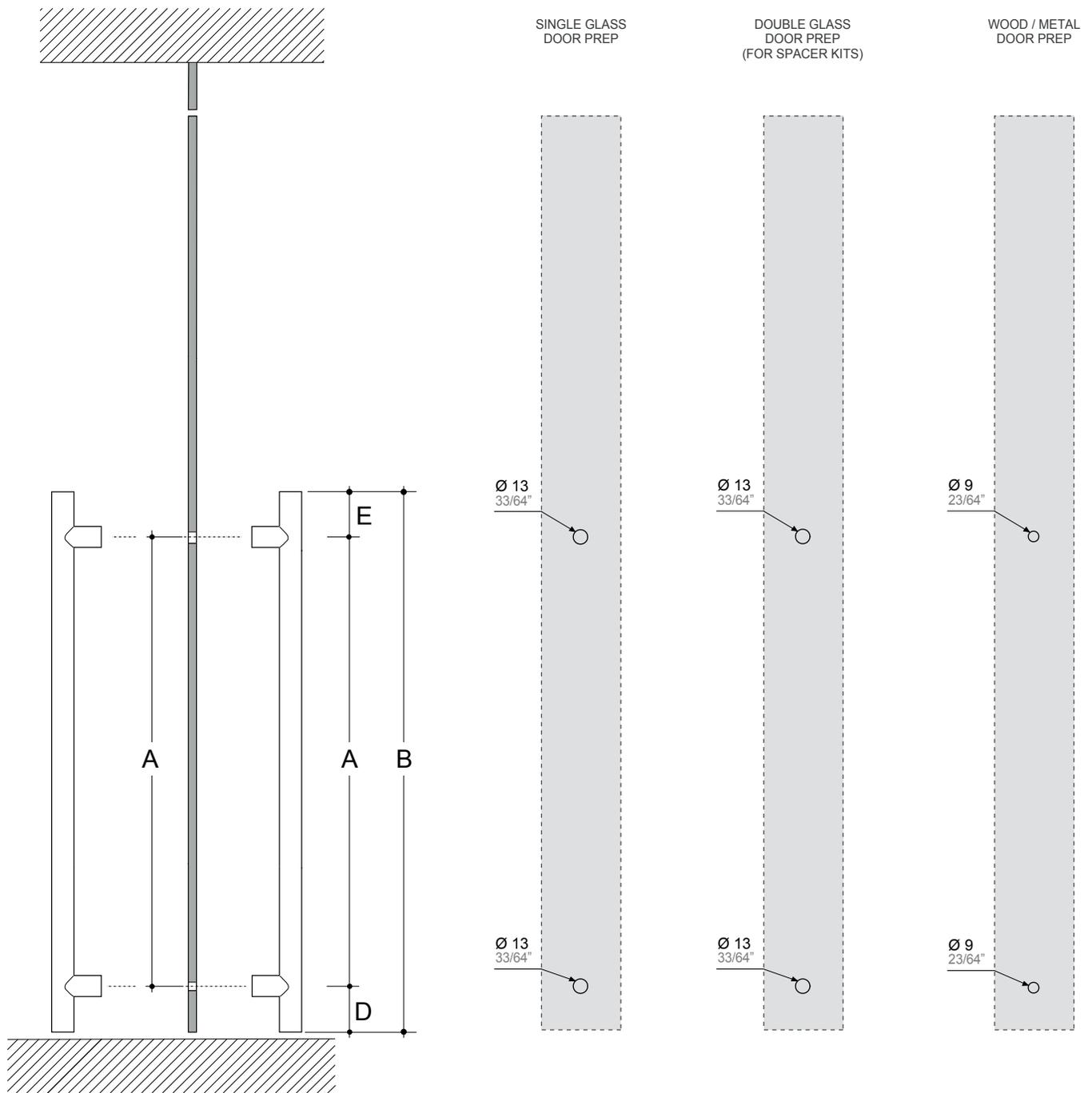
CONFIGURATION TO COMPLY ADA STANDARD (254 mm - 10" clearance from the floor)
